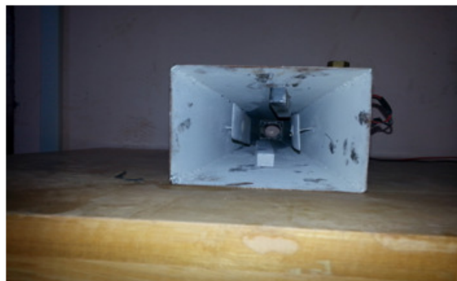
Figure 4: Placement of Magnets and Metallic plates in the MHD Generator.
